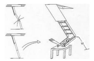
12. Add rubber feet to ladder and nail architrave timber to fit around the ceiling panel to conceal the cut of the opening. Mitre the corners. Fit architrave 2mm from edge inside edge of frame and allow clearance at the hinge end to prevent the panel clipping on the architrave when the door is opened.
