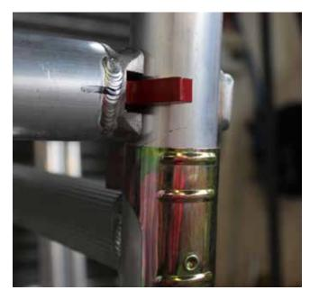
6. Standing inside the tower, position the platform on the top rung of the second 1m frame and secure wind locks (see photo)
