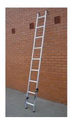
The ladder **must** be positioned at approximately 75 degrees. (1 measure out for every 4 measures up)
